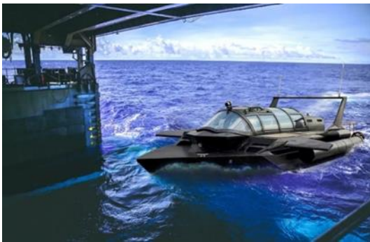
Fig. 8. Illustration FBS enters Patrol Vessel well-deck.
