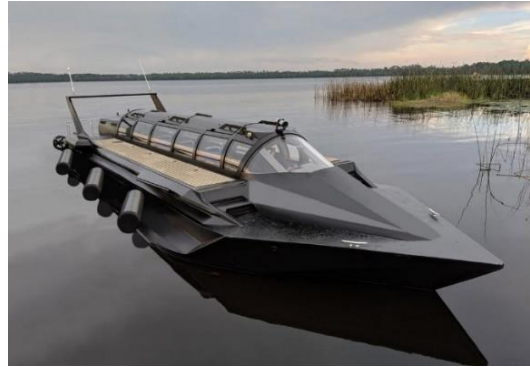
Fig. 10. Illustration of FBS with mini-torpedo payload.
